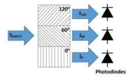
**Overview of three-channel PDM:** The light signal  $(S_{INPUT})$  is modulated for three data channels (polarization
