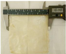
**Lab scale prototype** - membrane sample shows long term storage with no performance degradation (capacity or efficiency) over >500 hours of cycling.
