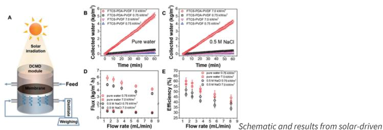
direct-contact membrane distillation (DCMD system) with FTCS-PDA-PVDF membrane
