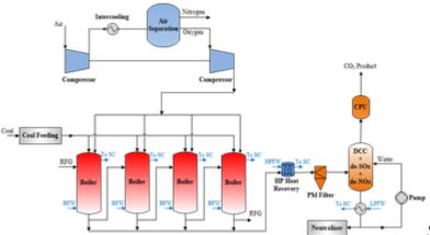
Simplified process flow diagram for an MPCC plant
