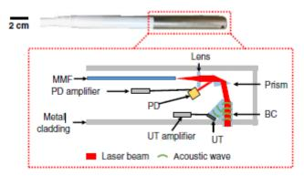
**PANIR system.** Photograph of a PANIR probe prototype and schematic drawing of the components (BC, beam combiner; MMF, multimode fiber; PD, calibrated photodiode; UT, ultrasonic transducer).
