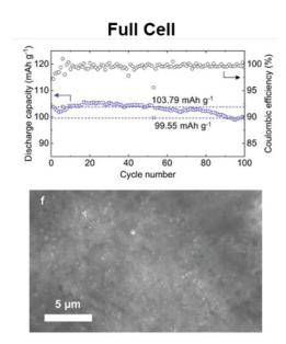
(Top) The discharge capacity and Coulombic efficiency of a full cell was calculated over 100 cycles. (Bottom) SEM images of the Na deposits were taken after 100 cycles.
